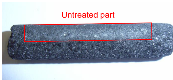
Figure 4.9.2: Incompletely treated graphite sample with the original sample holder
