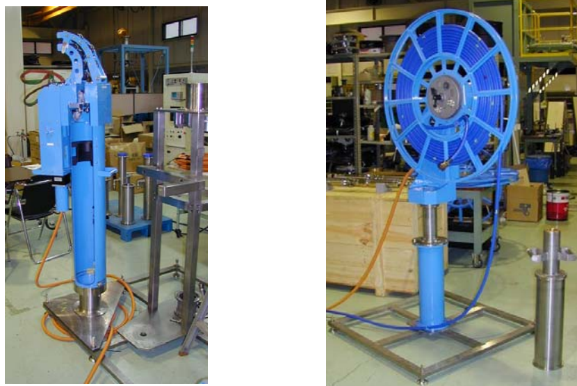
Figure 19 Equipment used to lower inspection devices in to an RBMK
