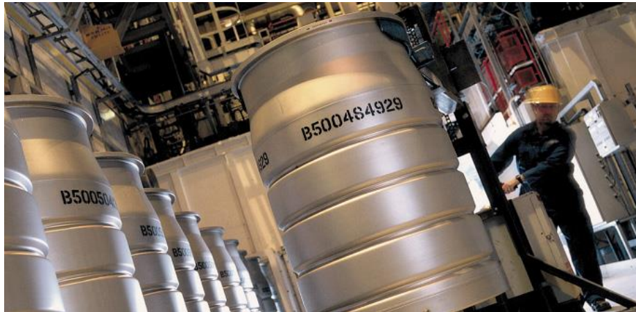
Figure 7 - 500 L ILW drum [11]
