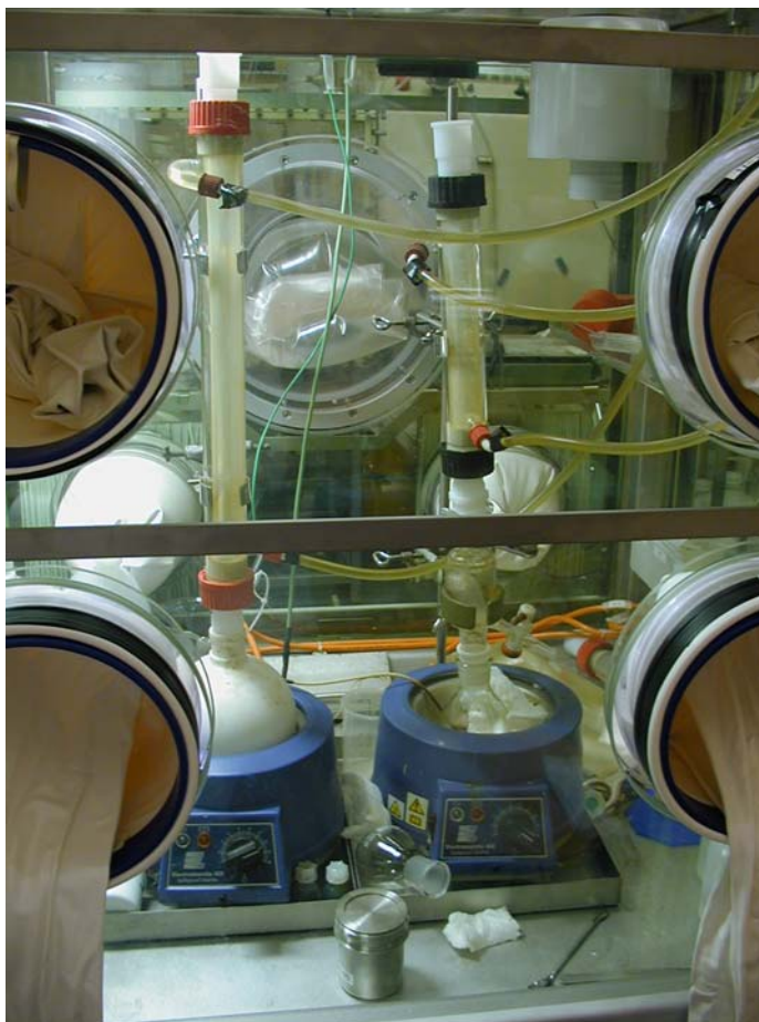
Figure 3.9: Pu dissolution (left) and denitration (right) facilities
