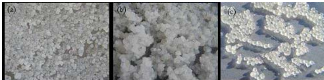
Figure 3.2: Kernels and agglomerates obtained with different heat transfer medium: (a) warm ammonia 4M, (b) C_2Cl_4 vapour and (c) silicone oil.
