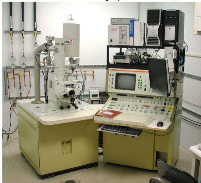
**Figure 3.7** Scanning Electron Microscope: JEOL mod JSM-840
