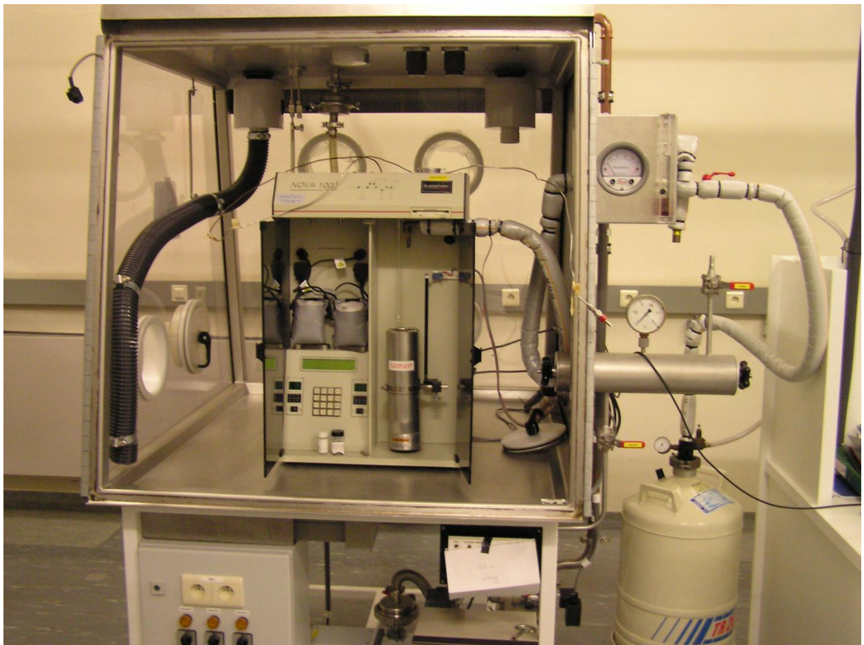
Figure 1. BET equipment for the measurement of the specific surface area of irradiated graphite.
