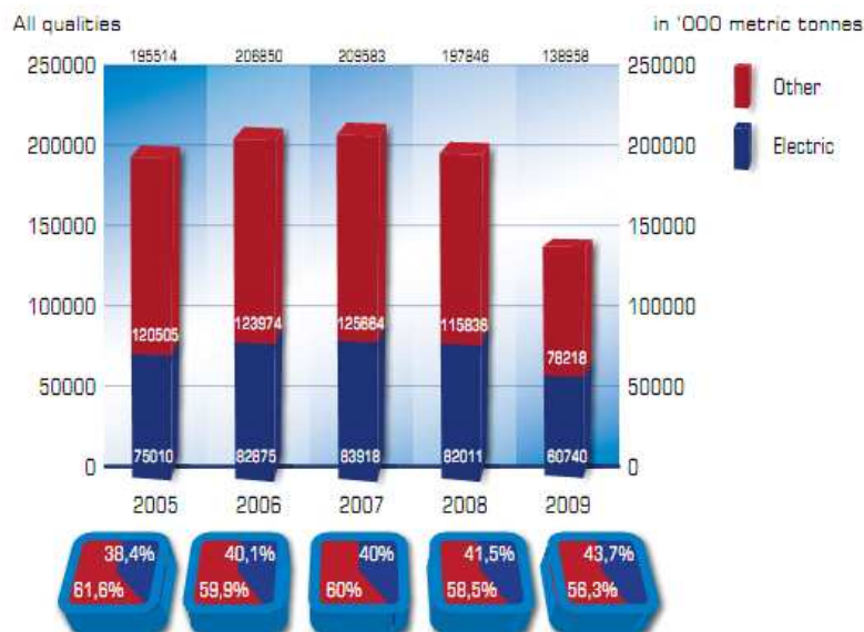
Figure 3.5.2-3 Crude steel production by process (Source: EUROFER 2010)
