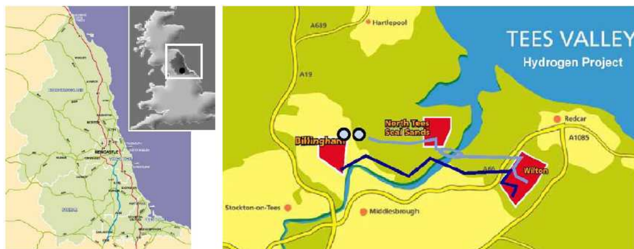
Figure 3.3.1-9 Hydrogen pipeline network operated by Linde in the UK (Source Roads2HyCom 2007c)
