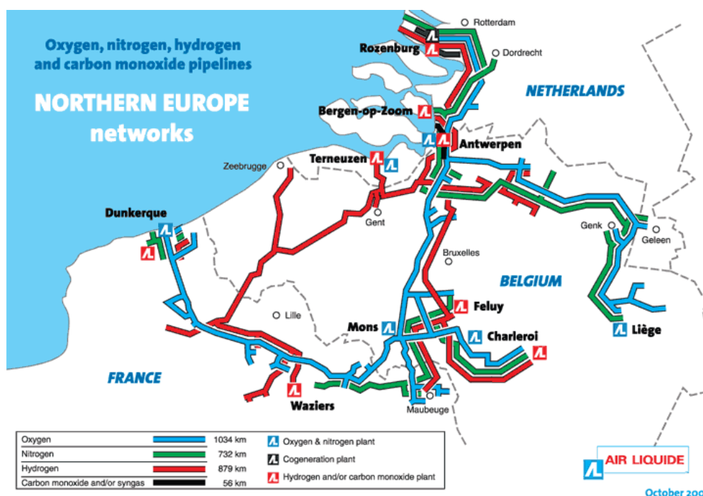
Figure 3.3.2-1 Air Liquide's oxygen, nitrogen hydrogen and carbon monoxide pipeline networks in Northern Europe (Source: Air Liquide)
