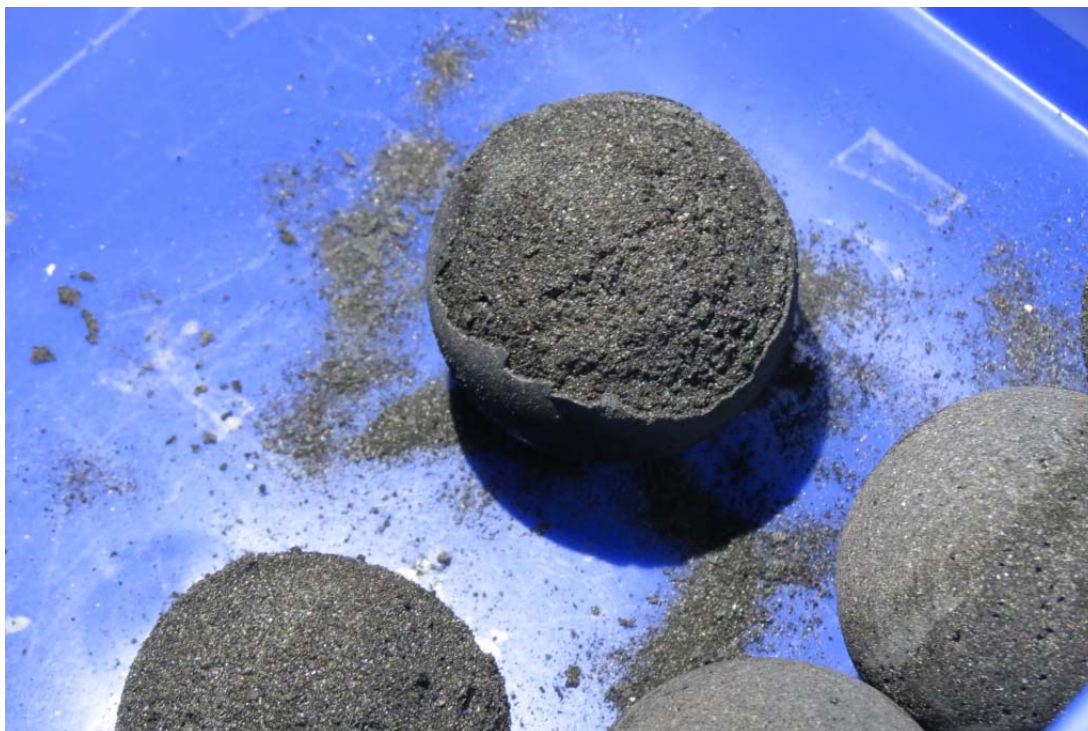
Figure 56: Pebble of lower layer after oxidation
