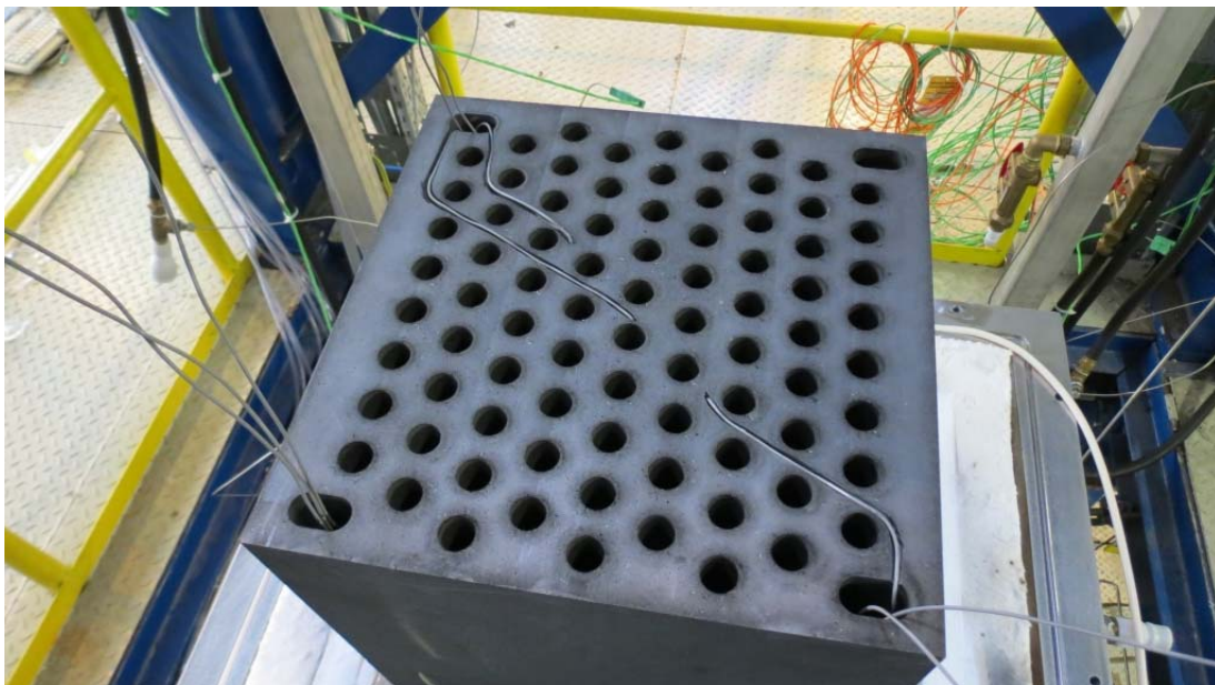
Figure 39: Block 5.1 after oxidation
