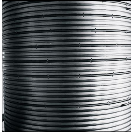
Figure 58: Cylinder with heating coils
