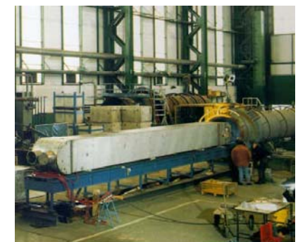
Figure 11.3 : Packinox heat exchanger and its shell
