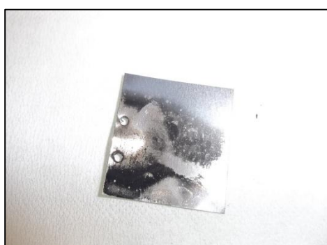
Figure 12: black deposit on the nickel foil (foil not irradiated)
