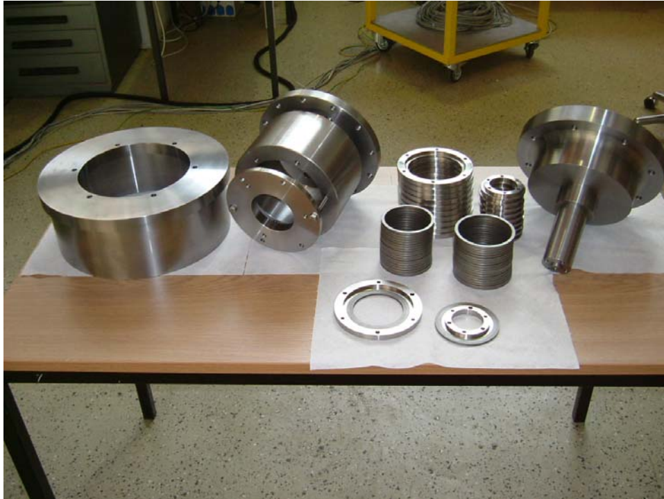
Fig.3 Components of the PMB, FLP500 shaft extension and bearing support
