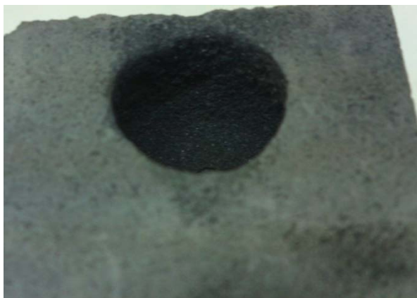
Figure 5.1: Manufacturing of graphite crucibles for molten salt applications using chemical etching technology
