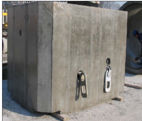
Figure 20 : Prototype of concrete package for irradiated graphite disposal : Total weight 24 tons - External volume 9.2 m 3 .
