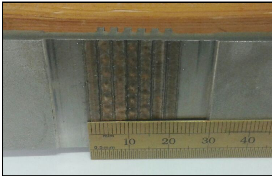
Fig. 18 The length of the weld mid-section gauge length. Note in this picture it exceeds 20mm and is ~22mm.
