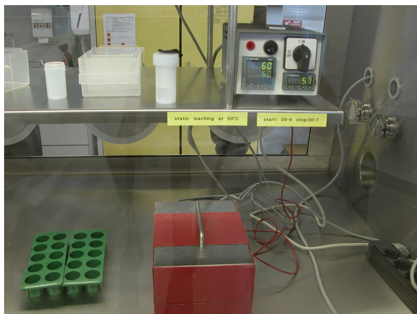
Figure 7: Argon-filled glove box for corrosion studies under inert atmosphere – running tests at elevated temperature
