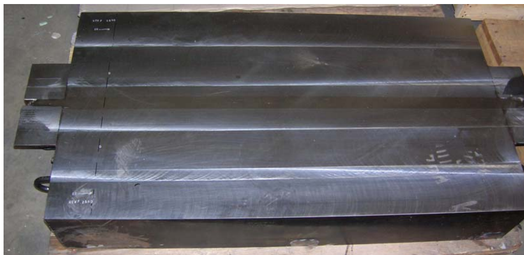
Figure 2-5 Welded plate used for Ageing tests
