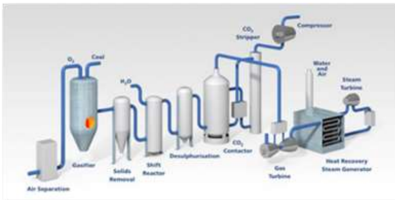
Figure 2-4. Pre-combustion process (CCSa, 2015)
