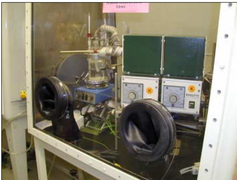
Figure 4.1: Thermal reactor for graphite treatment in a glove box
