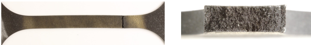
Figure 4-6: Macro shot of ruptured thin sheet specimen C7 (A800 H, 850°C, t_u = 16622 h)
