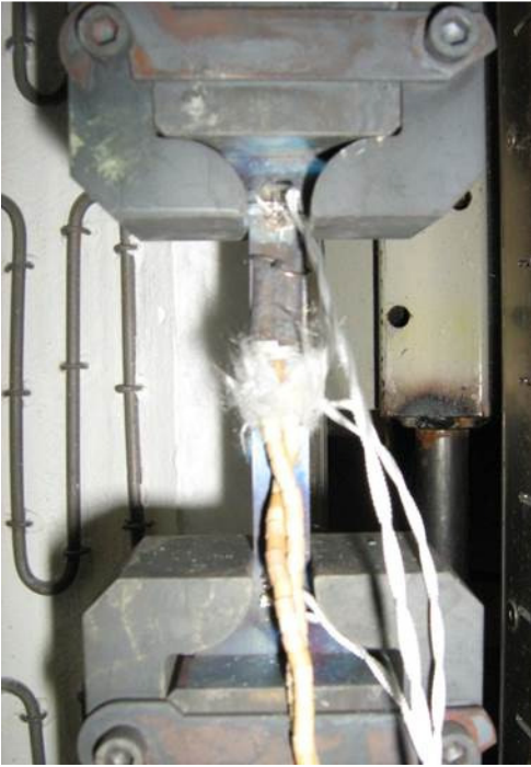
Figure 3-2: Shoulder support of specimen for tensile and relaxation tests
