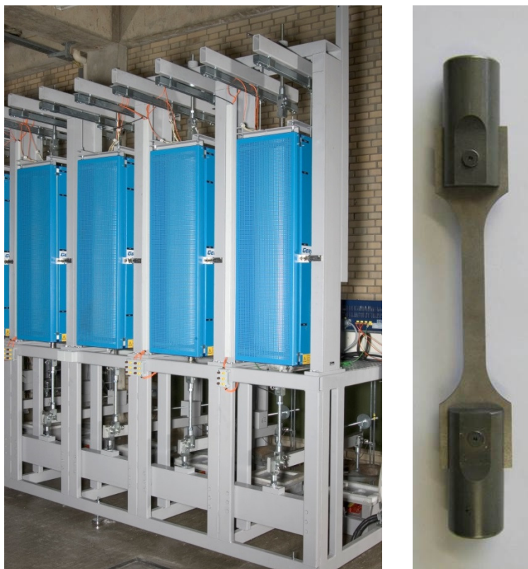
Figure 4-1: Multi-specimen creep testing machine for two in-line arranged sheet metal specimens
